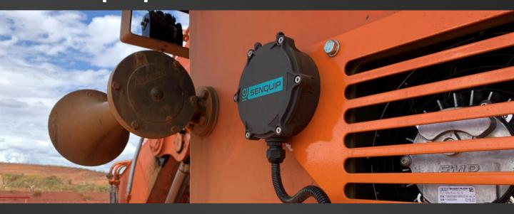
Senquip manufactures rugged, programmable telemetry devices that connect to industrial sensors and systems and send the data measured to the Senquip Portal or a server of your choice.
